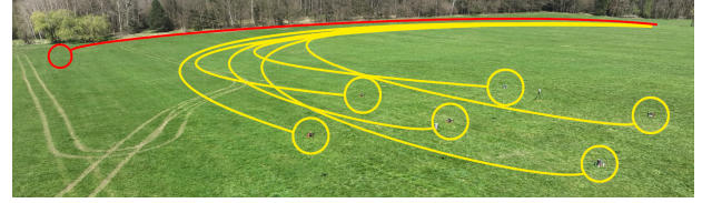
(c) A swarm of six UAVs (yellow) using the proposed approach. The group velocity of 5 \text{ m s}^{-1} was reached, while the swarm stayed coherent without reliance on GNSS and communication.
